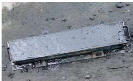
Fig No:6.4.3 A) After Placing Of Concrete in mould
