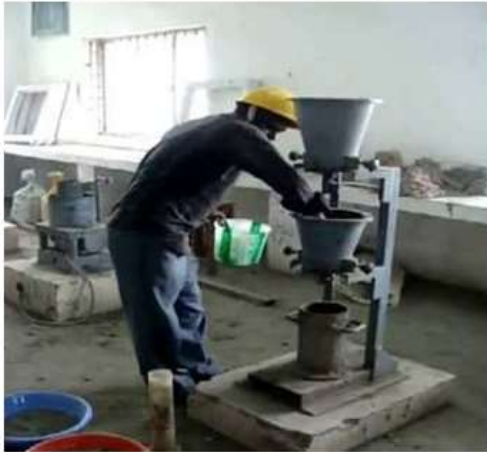
FIG NO: 6.1.2 COMPACTION FACTOR TEST
